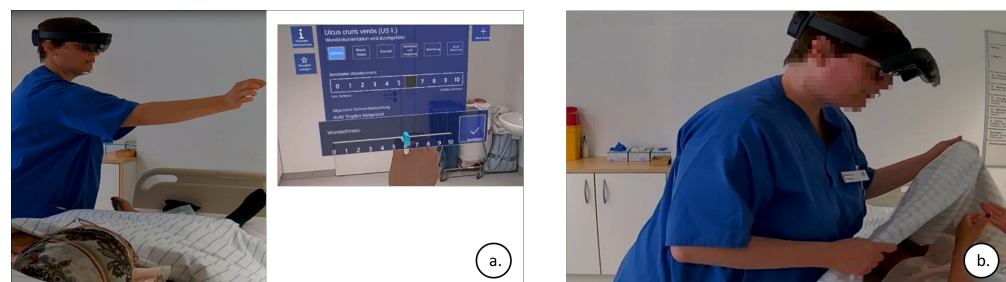
Figure 4. Special work situations at the bedside with the HoloLens 2: (a) Participant reaches over the patient to interact with the system by near gestures. (b) Participants raises visor to maintain eye contact with the patient.
