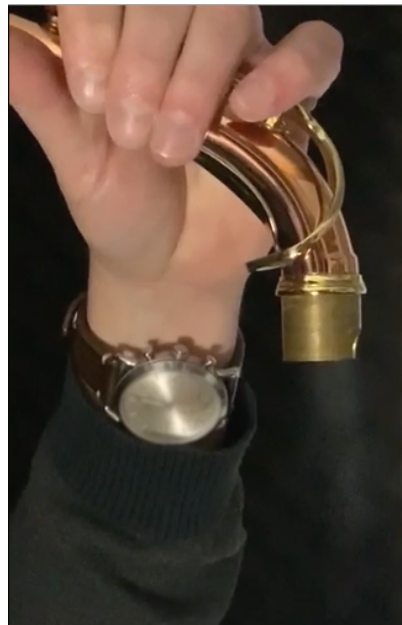
Figure 6. Smoke blown in alto saxophone mouthpiece and neck.
