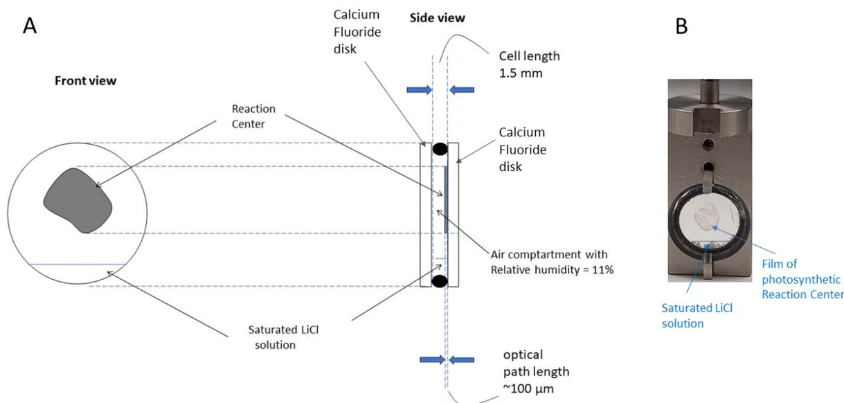
**Figure 2.** (A) Scheme of the sample compartment for FTIR experiments. (B) Picture of the sample compartment. See text for further details.
