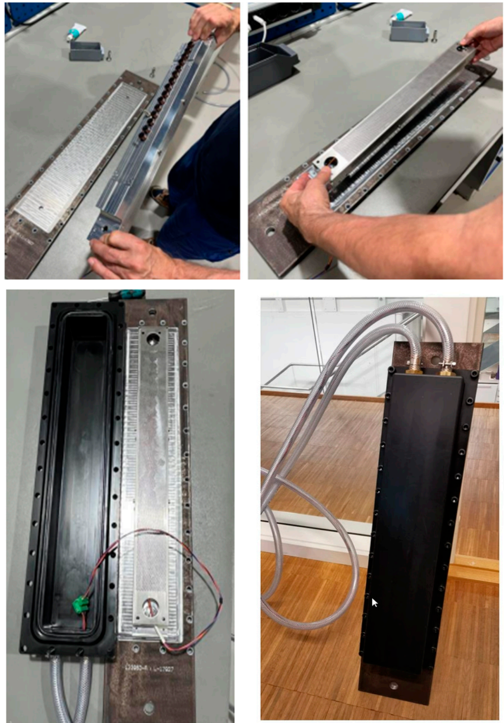
Figure 3. Test plate with sensors attached and protected from seawater.
