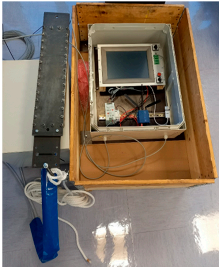
Figure 5. Equipment for thickness measurement of steel plate and remote sending that data.
