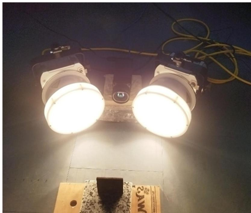
**Figure 3.** Illustration of the experimental setup used for FMTWI.
