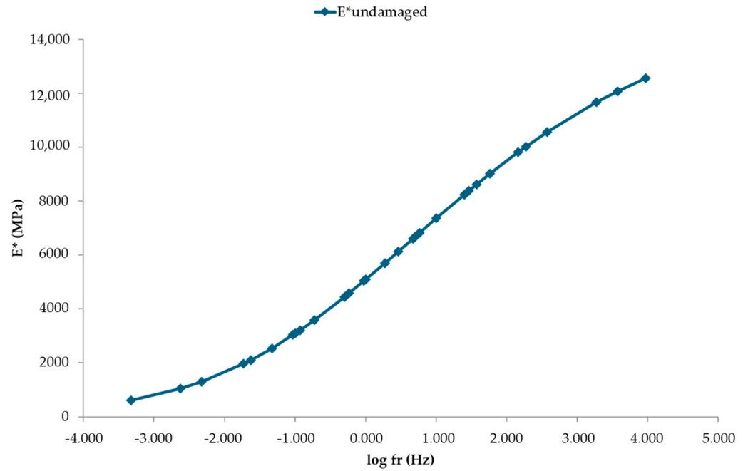
**Figure 7.** Undamaged HMA E\* master curve.
