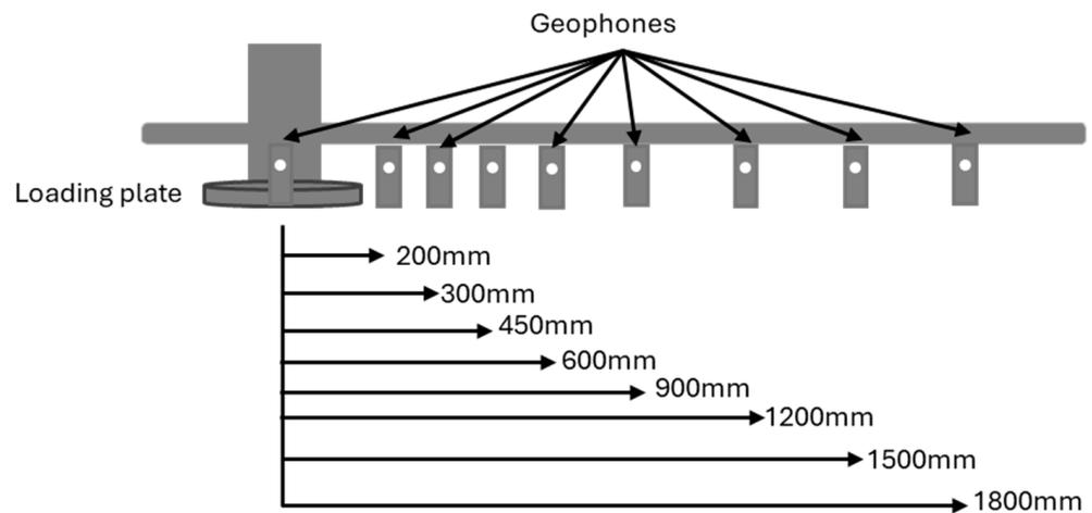
Figure 4. FWD deflection sensors set up.
