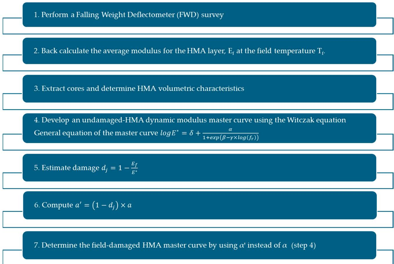
**Figure 1.** MEPDG methodology for  $E^*$  field-damaged master curve.
