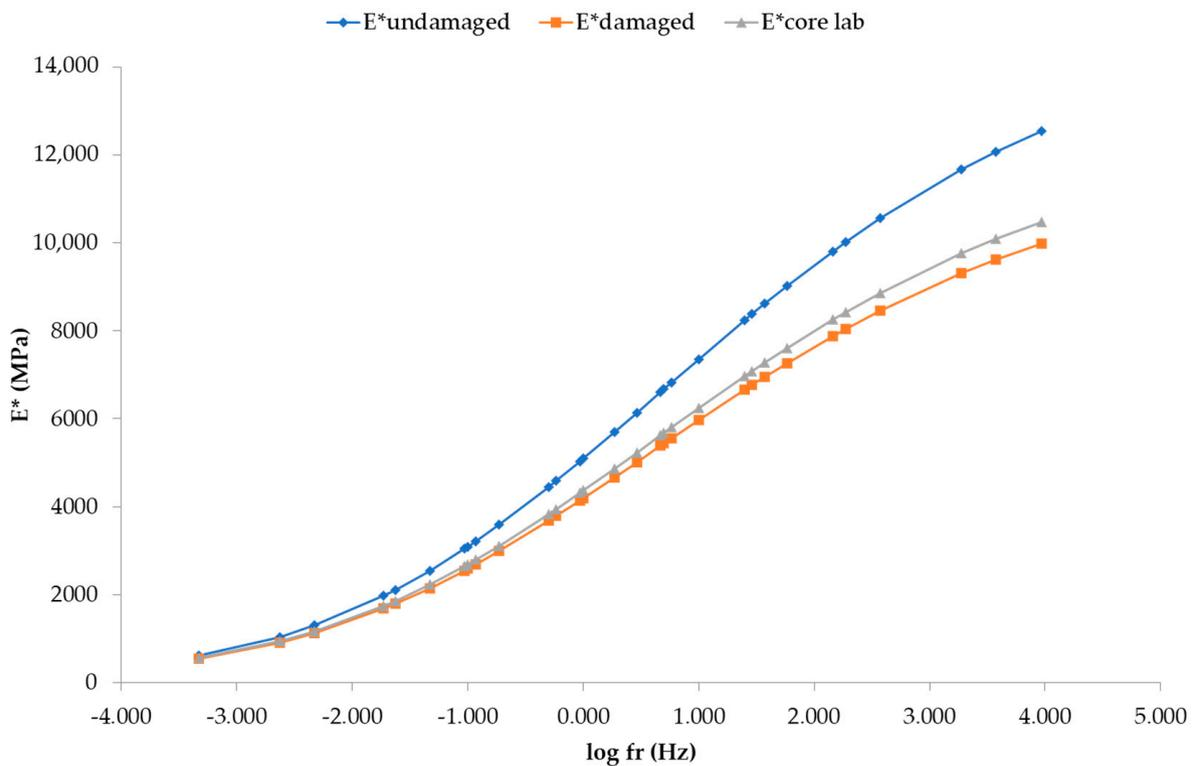
Figure 10. E\*undamaged, E\*field and E\*core master curves.
