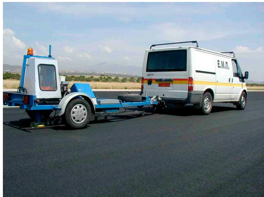
Figure 2. FWD measurements.
