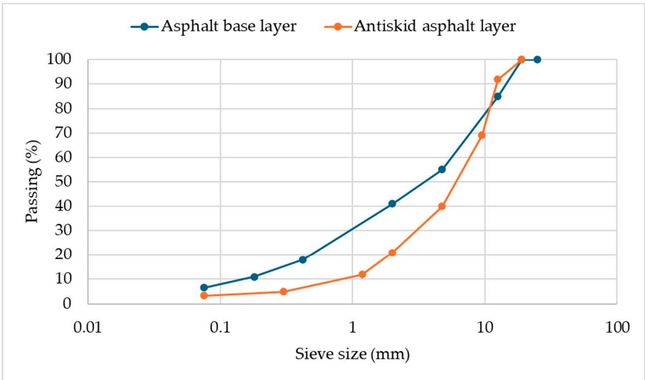
Figure 5. Aggregate gradation of the asphalt layers.
