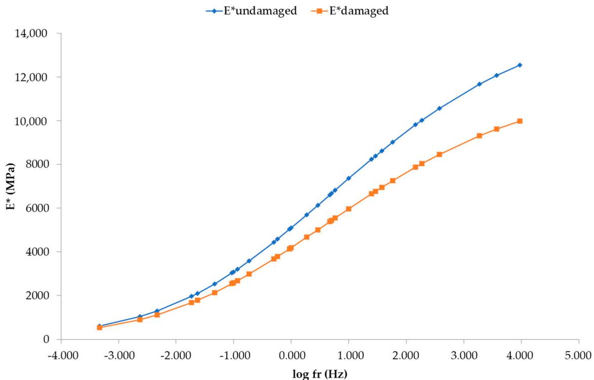
Figure 9.  $E^*$ undamaged and  $E^*$ field master curves.
