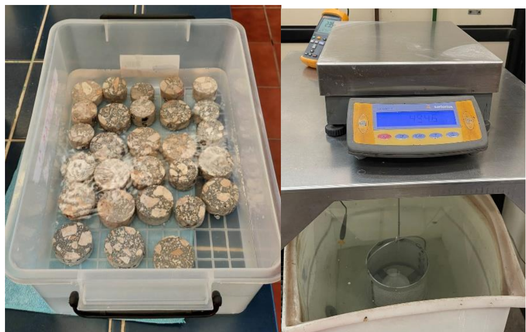
Figure 4. Determination of saturated and submerged weight by using a hydrostatic scale.
