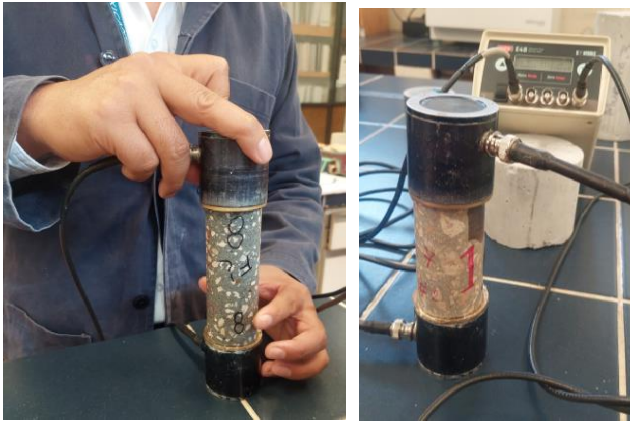
Figure 2. Representative pictures of the UPV measurement of unsaturated concrete cores.
