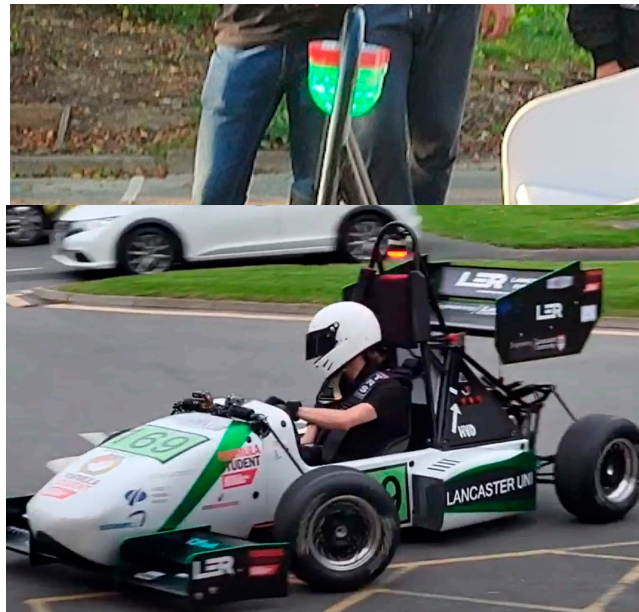
Figure 38. TSAL green and red lights inspection.
