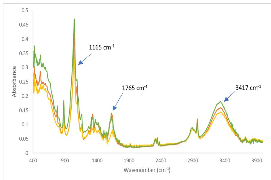
**Figure 3.** FTIR graphic for tangential cut of *E. bosistoana*: green line is 180 min, 2% NaClO<sub>2</sub>; red line is 180 min, 3.5% NaClO<sub>2</sub>; orange line 300 min, 3.5% NaClO<sub>2</sub>.
