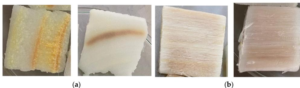
**Figure 1.** Samples bleached with  $\text{H}_2\text{O}_2$  after delignification: (a) *P. taeda* and (b) *E. bosistoana*.
