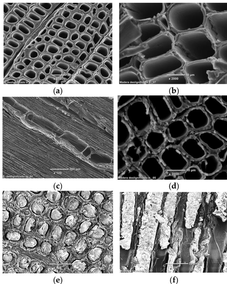
**Figure 2.** Cut wood: (a) cut crosswise normal pine wood, (b) cut crosswise delignified pine wood, (c) cut lengthwise delignified eucalyptus wood, (d) cut crosswise delignified eucalyptus wood, (e) cut crosswise pine wood impregnated with epoxy resin, (f) cut lengthwise eucalyptus wood impregnated with epoxy resin.
