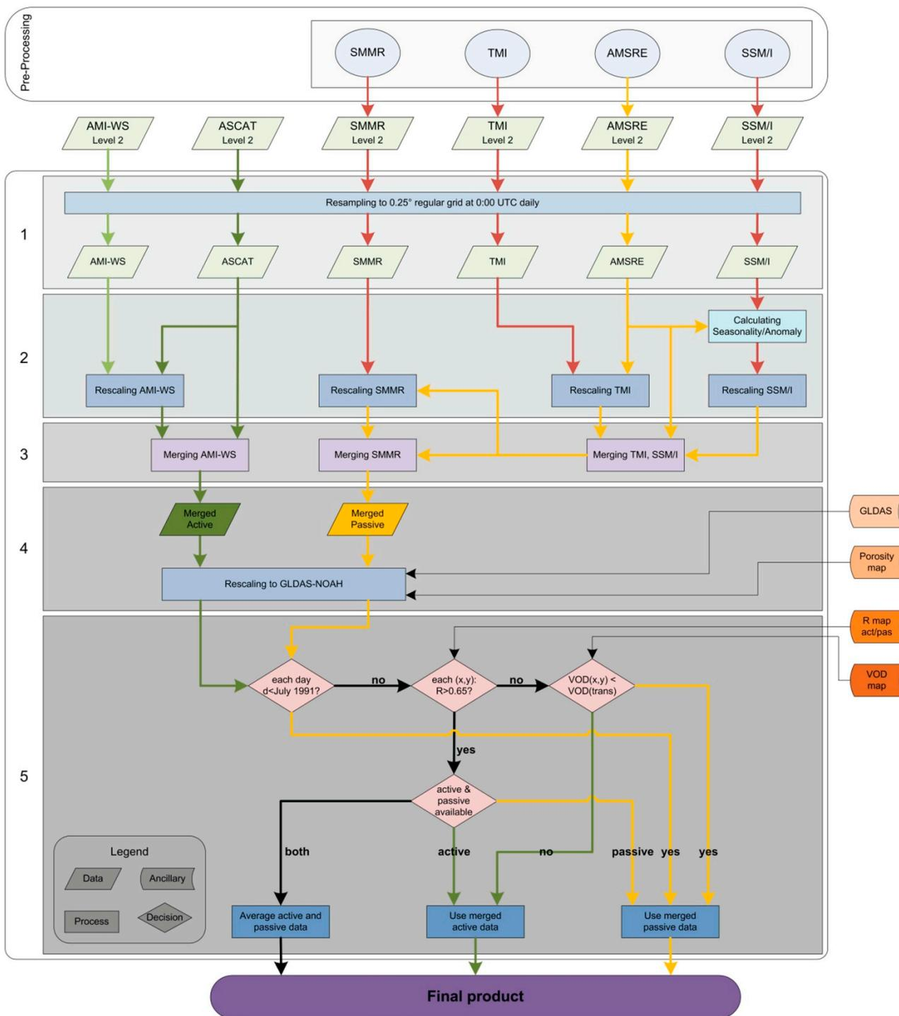
Note: Flow chart describing the process used to generate the global ECC SM product by using active and passive microwave sensors. Credit: Wolfgang Wagner, TUW. For a detailed explanation please refer to the published paper and to the cited works.
